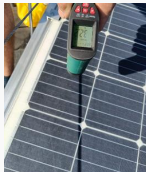
Figure 4: Temperature measurement of a section of a PV cell in the sun, using an infrared laser thermometer
