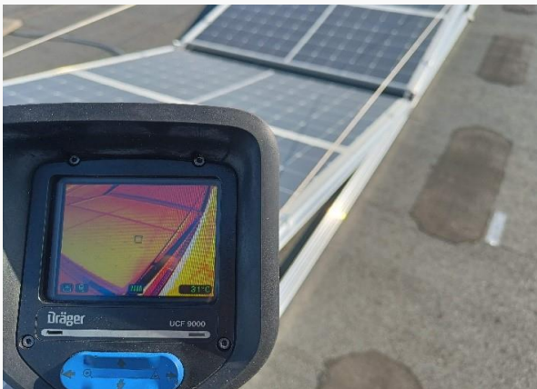
Figure 1: picture of the RABLE test setup including thermal imaging camera
