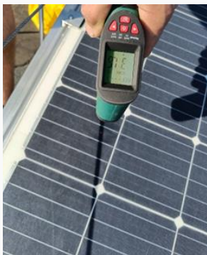
Figure 3: Temperature measurement of a section of a PV cell in the shade, using infrared laser thermometer
