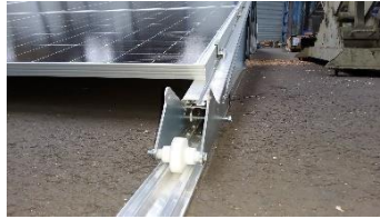
img. 4 setup of guidance bearings
