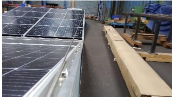
img. 3 setup of steel cable
